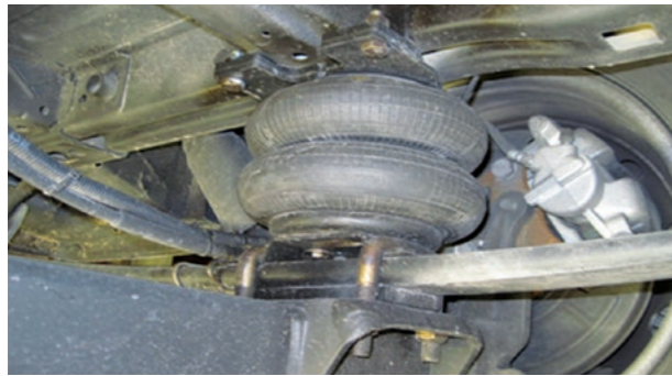
Light traces of oil (no dripping)
