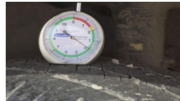
Tyres: Base of groove depth < 5 mm Note: The wear of the tyres is measured in the most worn groove on the tyre.
