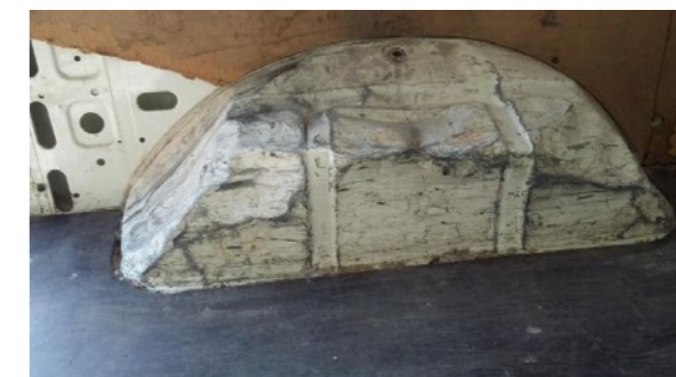
🔄 Internal deformations: Perforations, cuts, deformations beyond economic repair. Denaturing and uncorrectable deposit (powder, paint, etc.) (Wheel arch not recoverable if repair time > 3h)
