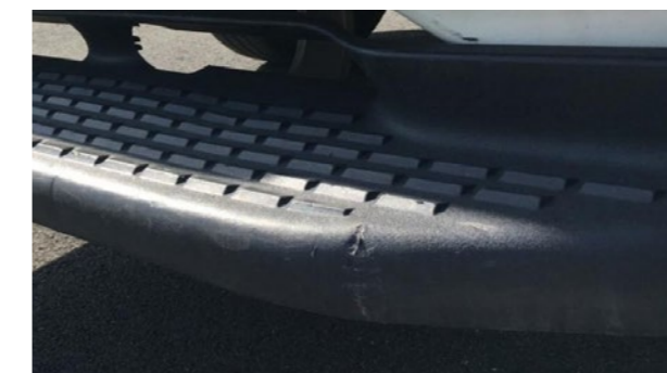
🔧 Rear footboards: Deformations within economic repair
