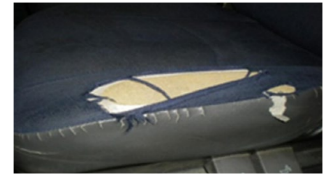
🔄 Burn > 3 mm, perforation or tear in the cover, without deterioration of the foam
